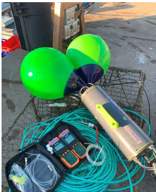
Figure 3. LiftLabs inshore acoustic-inflate system.
