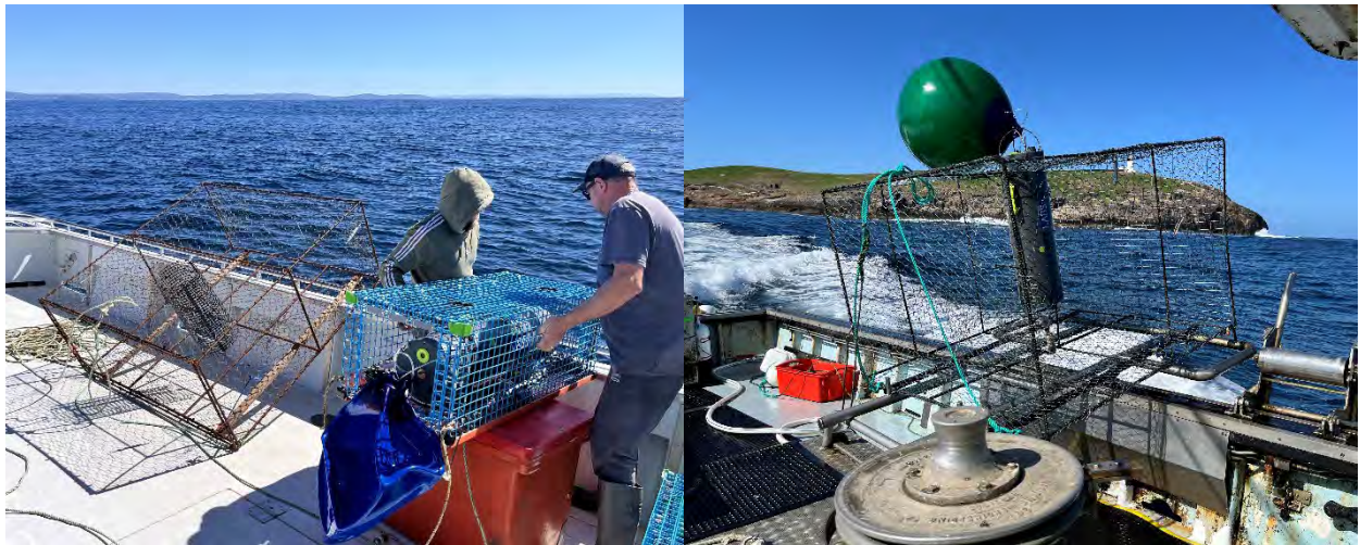
Figure 4. LiftLabs offshore acoustic-inflate system: Sled configuration (right) and centre trap-mounted configuration (left).
