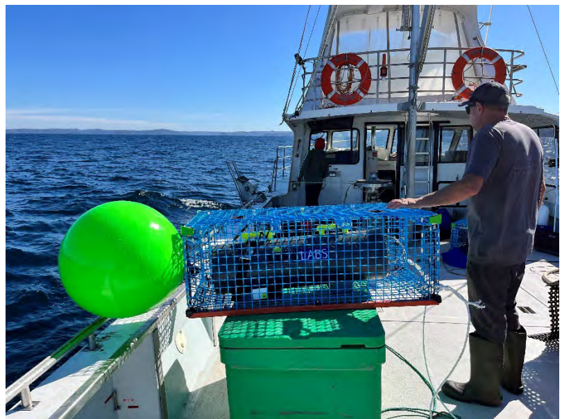
Figure 9. Offshore Lift system protective cage, configured as a separate sled.
