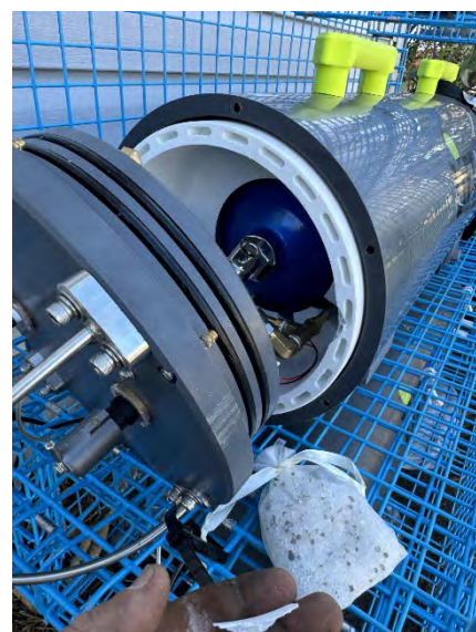
Figure 11. Fisher 2's imploded Offshore Lift canister.
