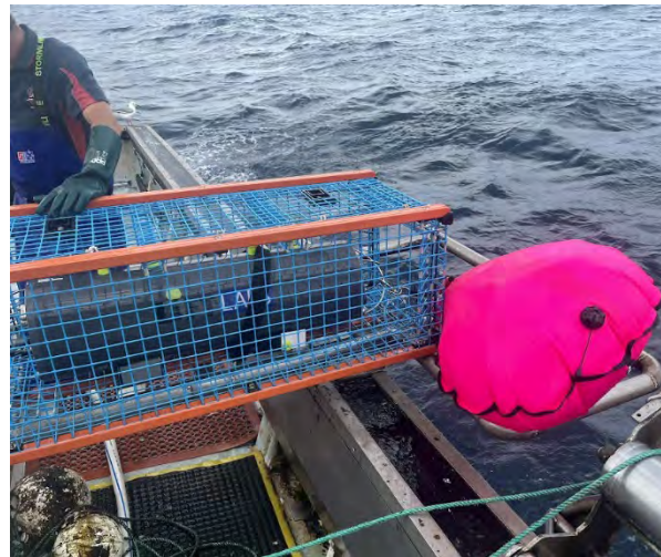
Figure 14. Updated Offshore Lift option with easily detachable lift bag buoy.
