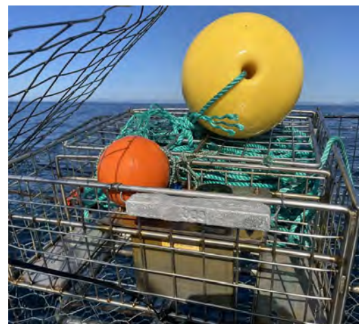
Figure 6. (a) Rust challenges with Ashored MOBI system; (b) Zinc anode attached to Ashored cage
