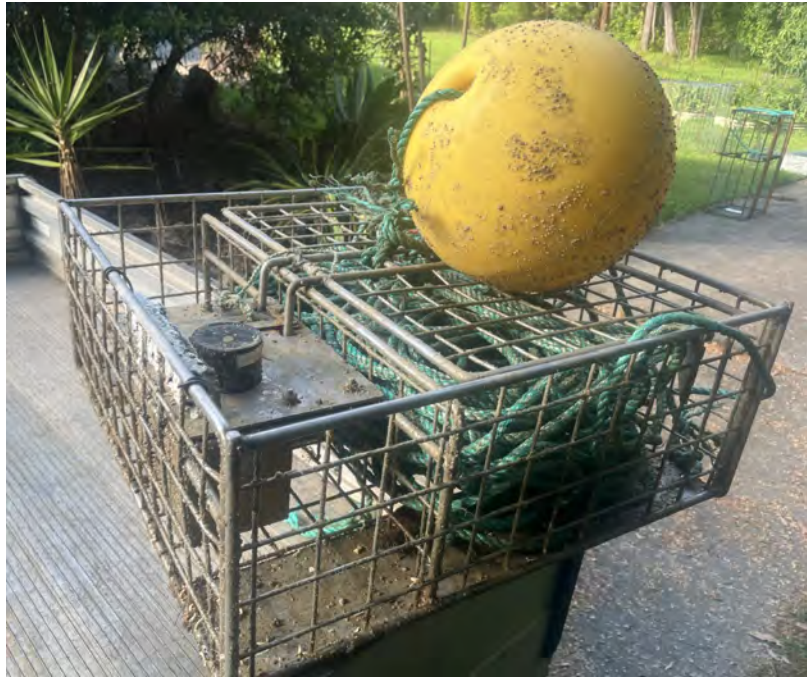
Figure 7. Barnacle-covered Ashored MOBI cage and buoy.
