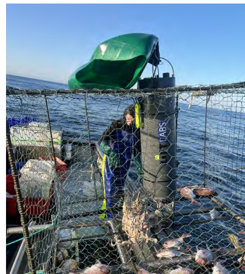
Figure 13. Offshore Lift mounted within fish trap with exploded buoy
