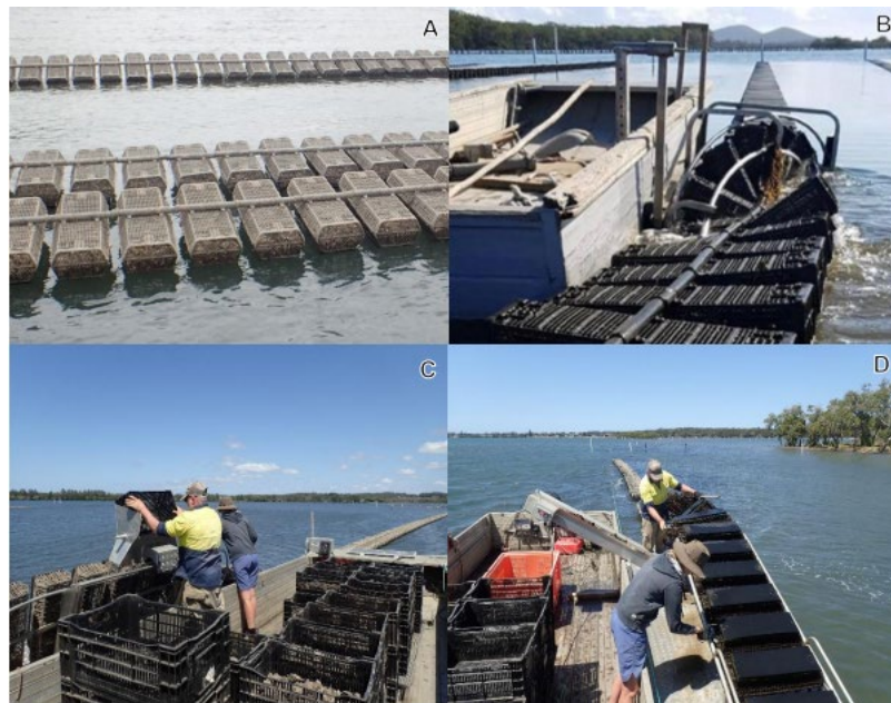
Figure 17. A FlipFarm system, in its drying configuration (A), in the process of being flipped by a mechanical attachment fixed to the oyster punt (B), being loaded in bulk with the assistance of an electric motor-driven line hauler (C), and being transferred back to bins using a conveyor belt (D). 16 .
