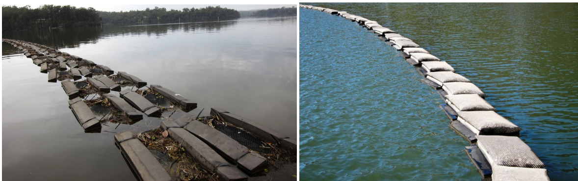
Figure 14. Another design with dual baskets and two floats per basket. This design requires the baskets to be manually flipped for drying as per the picture on the right. (OWA)
