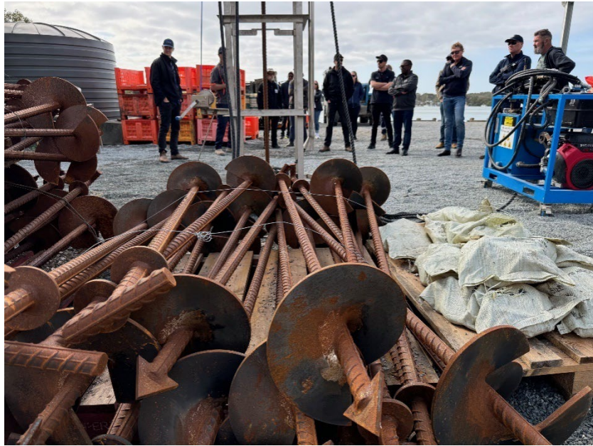
Figure 21. Use of a hydraulic drill and screw anchors provide up to 9 times the holding force of traditional block weights. (OWA)
