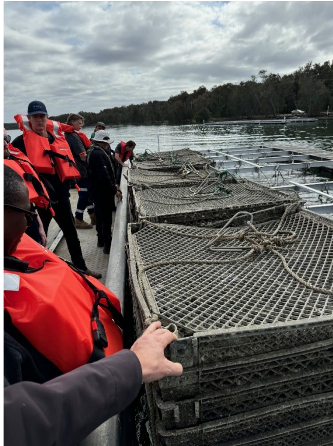
Figure 23. The new design constructed of aluminium with black blocks being examined during the 2024 NSW oyster conference field day. Note the existing trays with lids, which are raised for drying here, but usually hang below the raft in the water column. (OWA)
