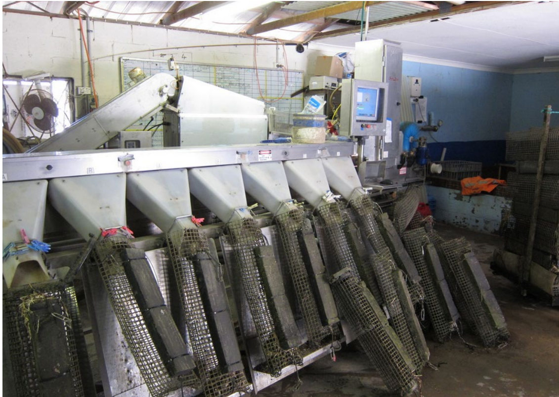
Figure 15. Mechanisation and advancements in technology have allowed graders to fill baskets far faster than by hand. This type of basket is kept closed with the use of an 'occy' strap. (OWA)
