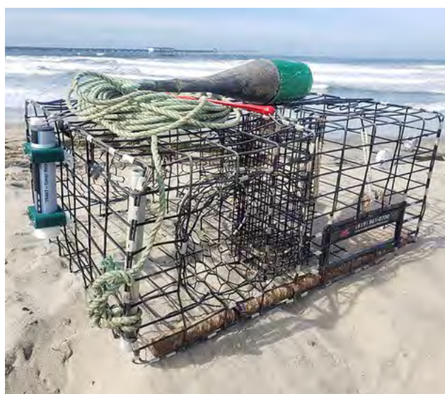
Sub Sea Sonics Time release system attached to trap (right) and with Guardian rope retrofit (left)
