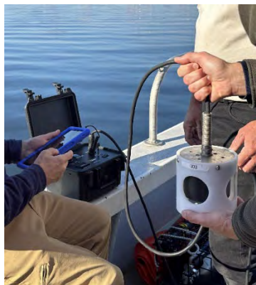
Over the side transducer system with associated deck box and tablet
