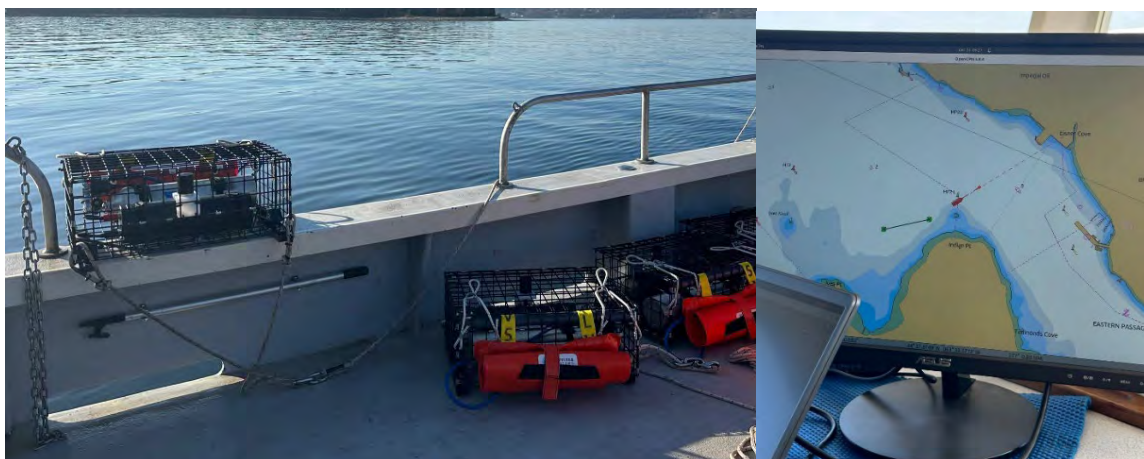
Left: Multiple lift bag anchor systems that would be attached to string of traps; Right: Single Ping Positioning system that shows where gear is located underwater (green dots)
