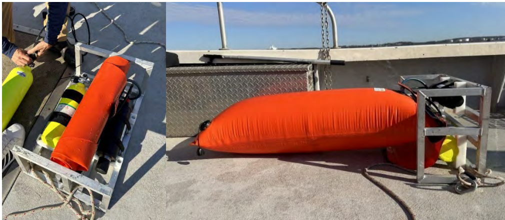
Lift bag systems that would be attached directly to traps or as an anchor on strings of traps
