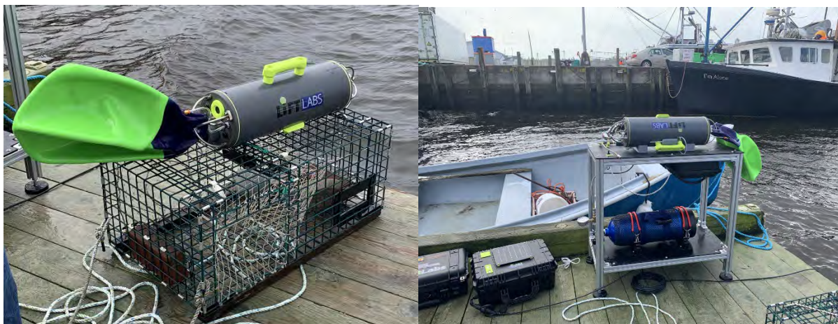
Left: LiftLabs system attached to trap; LiftLabs system refill setup (can customise to vessel needs)
