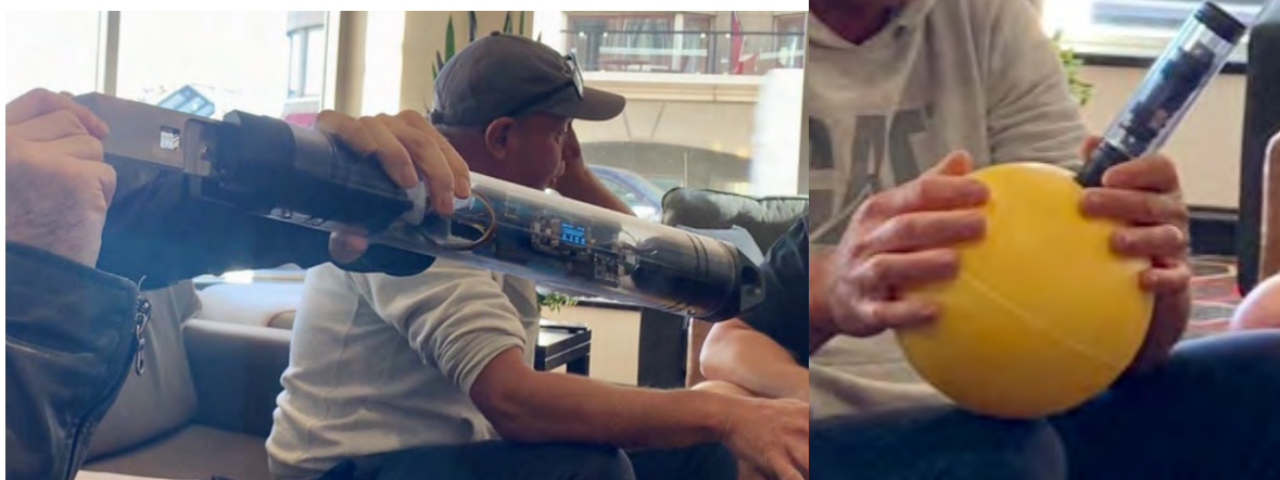
Left: Time release system; Right: GPS location device (can be added to buoy or gear)
