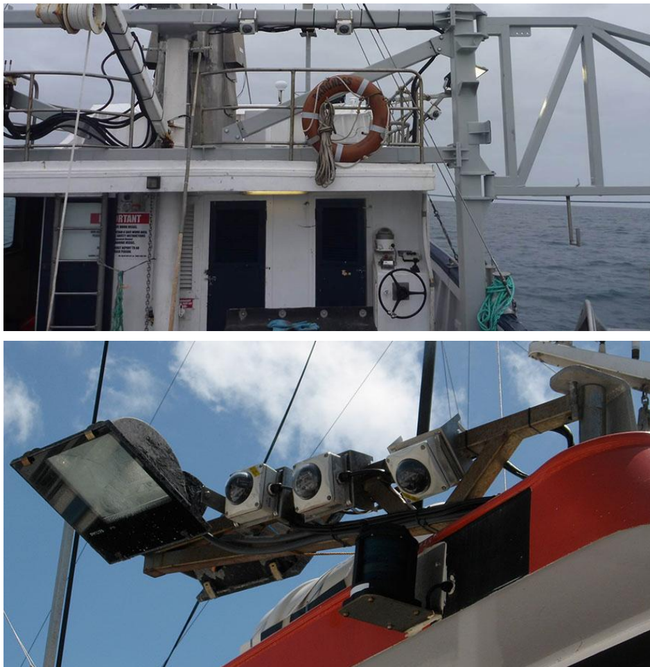
Figure 18. AFMA Electronic Monitoring System installed on a boat
