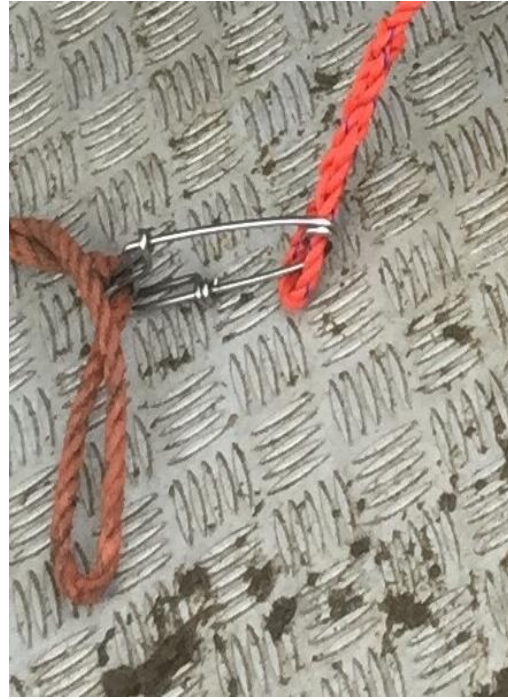
Packed rope bag attached to dan line with shark clip (NSW Lobster fishery example)
