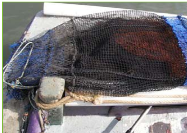
One type of BRD which is used by many prawn trawl fishing boats is the square mesh codend (part of the net where the catch collects). The square shape of the mesh means it remains open when it is full, allowing juvenile prawns and fish to escape, source: OceanWatch Australia
