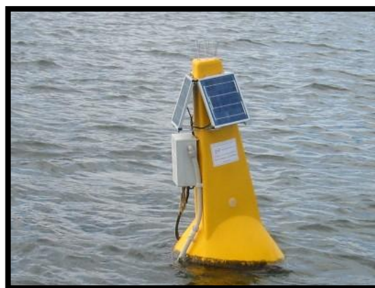
Figure 5. Water quality monitoring buoy in the Clyde River
