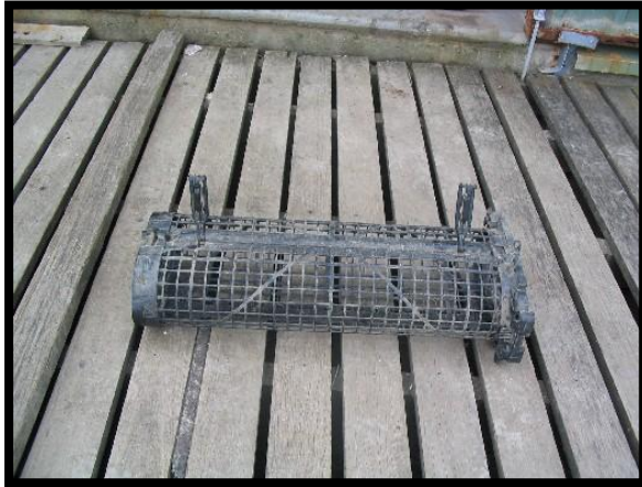
Figure 18. 'SEAPA' basket showing the fabricated plastic clips for attachment to long-lines
