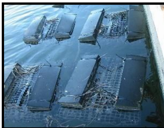
Figure 16. Polyurethane floatation attached to bags
