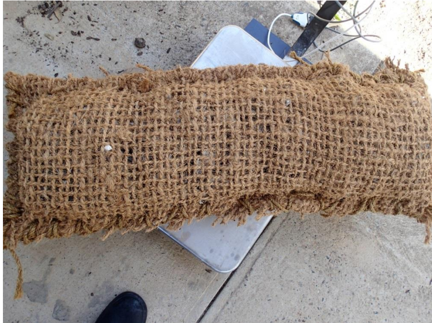
Figure 5-2: Example Single Oyster Shell Filled Bag
