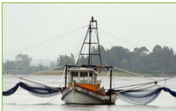
An Estuary Prawn Trawler working on the Clarence River, source: Debra Novak
