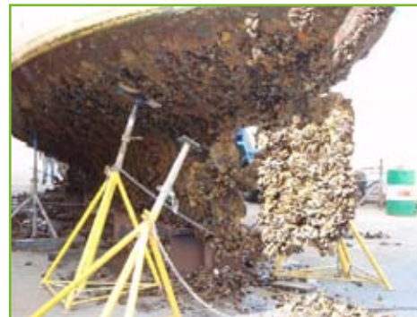
Marine growth can cause fouling of boats and other structures, source: Tasmanian Fishing Industry Council 2008
