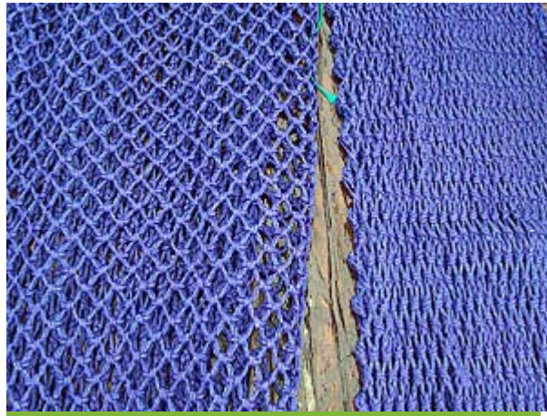
Photo: Rotated-mesh (T90) on left and standard diamond mesh on right.
