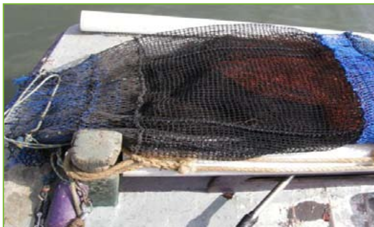
One type of BRD which is used by many prawn trawl fishing boats is the square mesh codend (part of the net where the catch collects). The square shape of the mesh means it remains open when it is full, allowing juvenile prawns and fish to escape, source: OceanWatch Australia
