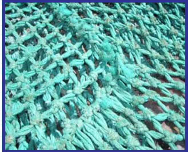
A codend with a square-mesh panel to facilitate the escape of small fish. This design may be superseded/ improved upon by the rotated mesh concept being developed.
