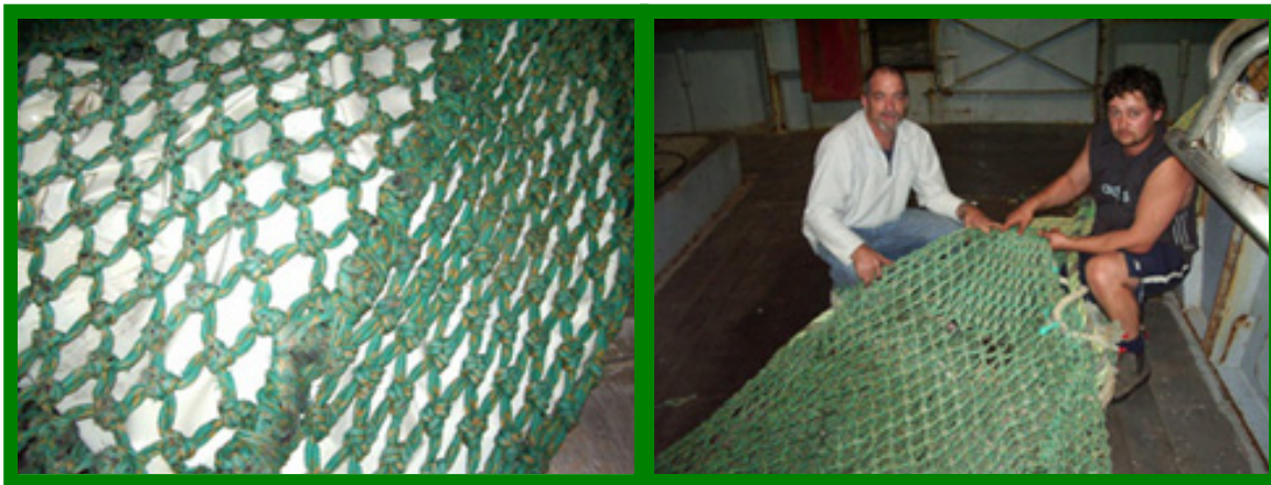
Left: Close-up showing a seam where the T90 panel is joined to the codend, note how the meshes are held open. Right: South-east trawl fishers with a modified T90 panel codend.
