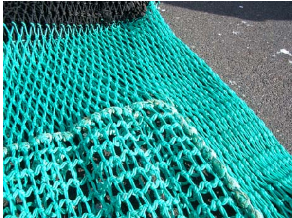
The square mesh panel has proven effective in reducing bycatch
