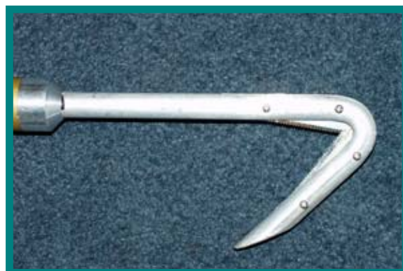
Head of a line-cutter showing the protective 'V' shaped blade
