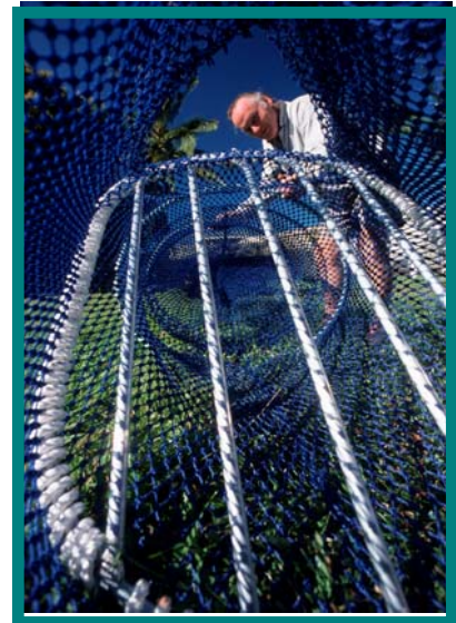
The Nordmore grid, probably the most well known bycatch reduction device.
