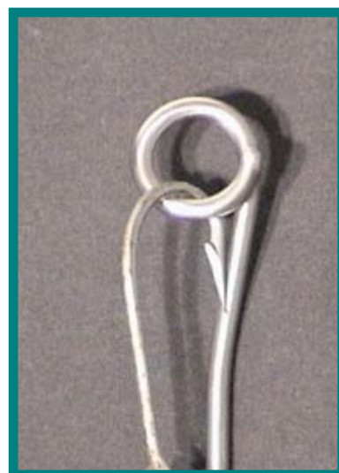
As the embedded hook is retrieved, the unique shape of the de-hooker prevents the hook from re-engaging.
