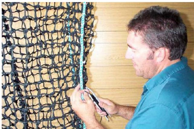
*This square mesh codend was used in a research charter in the Queensland scallop fishery in 2002. The 12mm polyethylene rope was used to take the weight of the catch, reducing knot slippage and distortion.*
