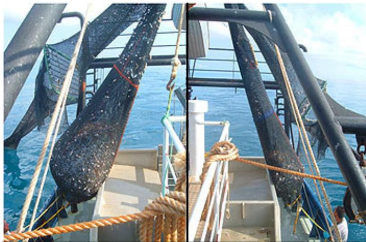
Photo: The net on the right has the 'popeye fishbox' BRD installed, the net on the left doesn't. The difference in amount of bycatch is quite obvious to the eye. Photo taken by Erik Raudzens (AFMA).
